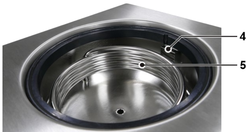
Fig. 2: Ice condenser chamber
