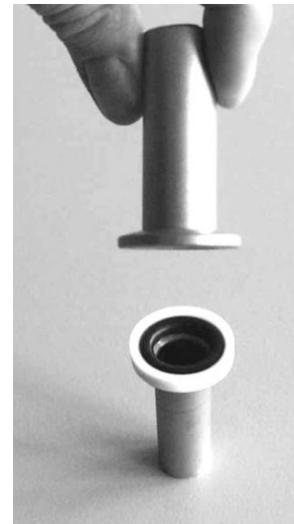
Fig. 57: Small flange with centring ring and small flange
