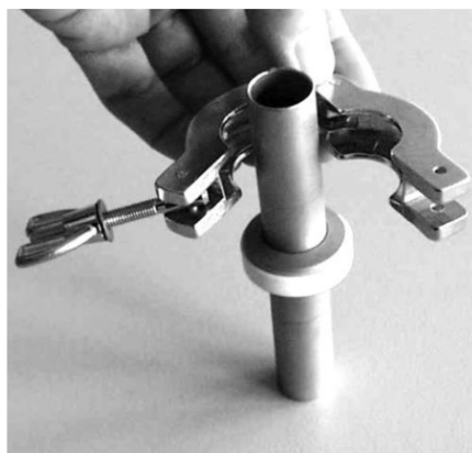
Fig. 58: Attaching the clamping ring
