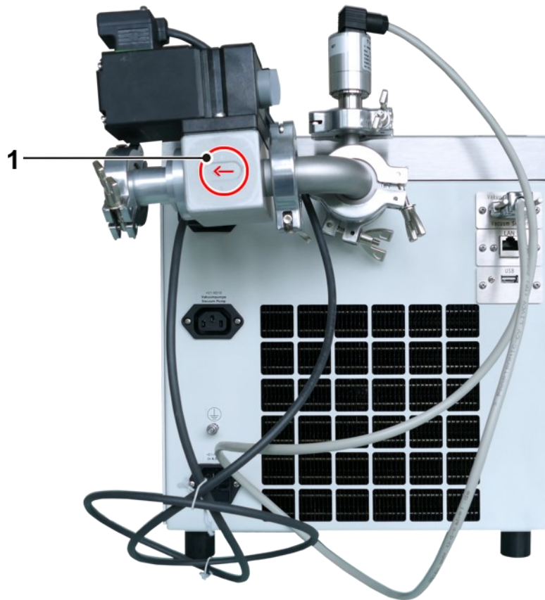
Fig. 18: Installation of the pressure control valve
