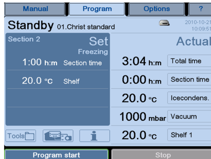
Fig. 71: The freeze-drying process can be started with the aid of the button "Program start".
